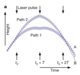
In spite of the small difference of heights between the 2 paths, the huge value of  $\omega_C$  provides the best test of Einstein's red shift
